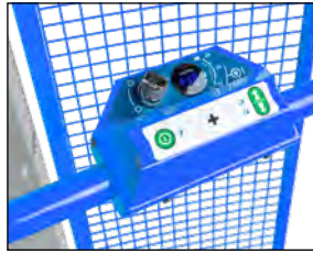
Lockout key & two-hand controls for safety
