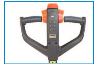
Pin can be set so only selected personnel can use the unit
